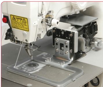
Full close step motor-controlled feeding plate
